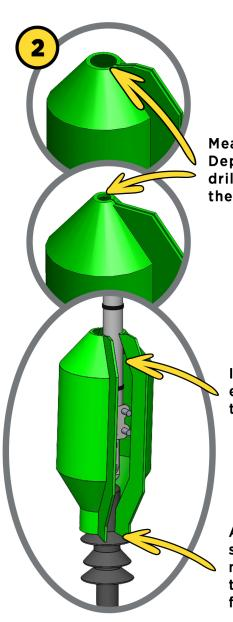
Measure wire. Depending on wire size, drill or trim the cone of the cover If conductor cover is used, ensure it is overlapped by Fasten cover the cover by a min. of 2" together
